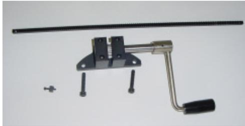
Check both the C075 column and the C001 gear housing casting to ascertain whether they have been properly machined to accept the installation of the C230 Height Adjustment Kit (see photo 1). If not, those parts can be ordered from the factory.
